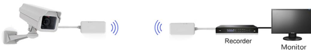
Solution Two Camera 1,2,3---Bridge Bridge---Recorder---Monitor
