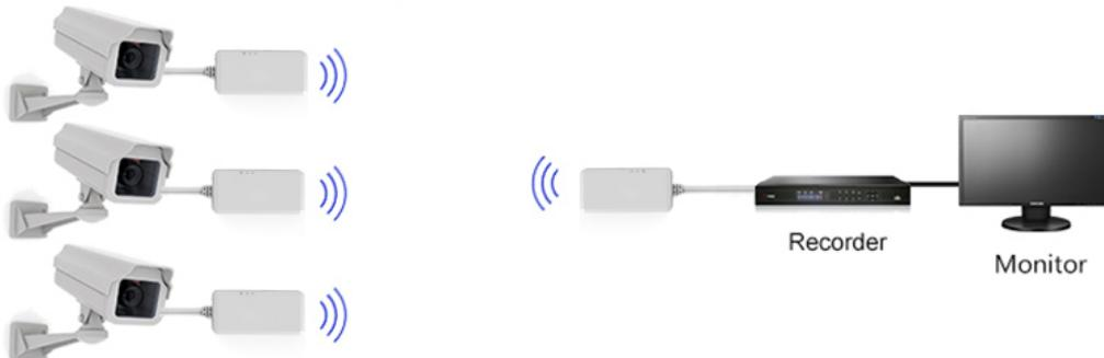
Solution Three Camera 1,2,3---Switch-Bridge Bridge---Recorder---Monitor
