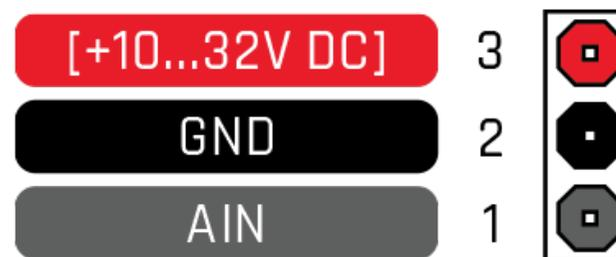
**Figure 2 MSP500 socket pinout**
