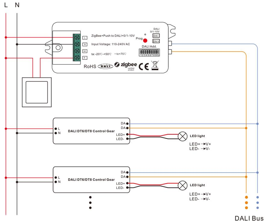
**Note:** Max. 50mA DALI bus PS output to supply control current to up to 25 control gears.
