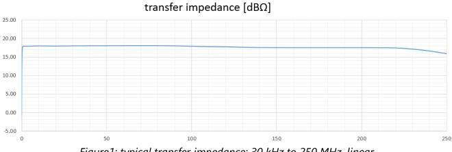
Figure 1: typical transfer impedance: 30 kHz to 250 MHz, linear
