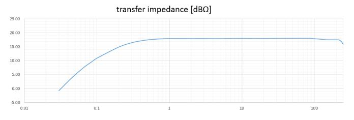
Figure2: typical transfer impedance: 30 kHz to 250 MHz, logarithmic
