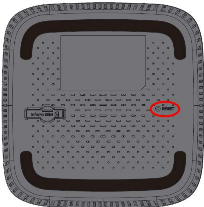
Figure 26 Micro SIM card slot and RESET button on the bottom panel (Nebula FWA510)
