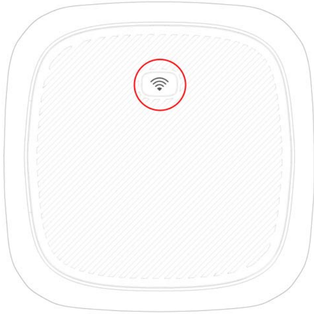
Figure 18 WPS and WiFi On/Off Button on the Top Panel (NR5101)
