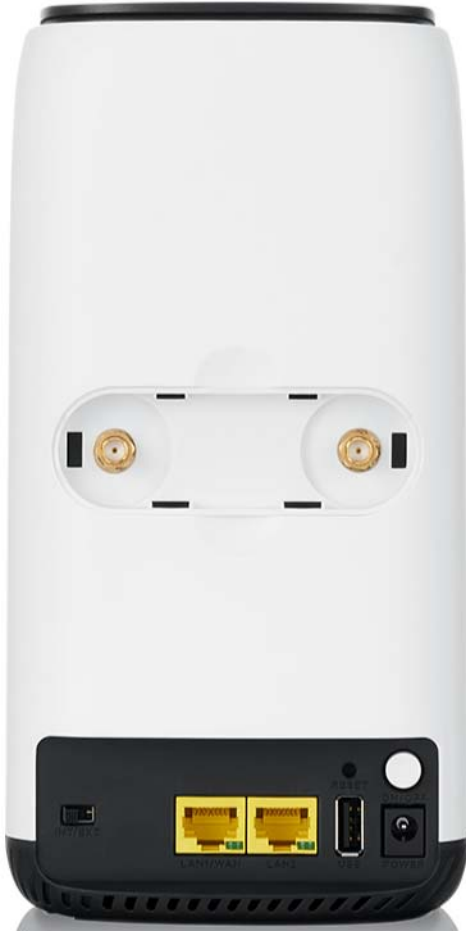
Figure 19 Antenna Ports on the Rear Panel (NR5101)
