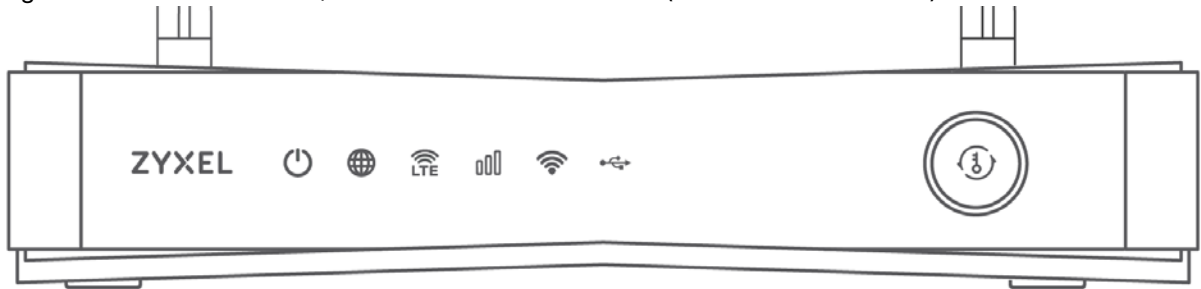
Figure 16 WPS and WiFi On/Off Button on the Front Panel (Nebula LTE3301-PLUS)
