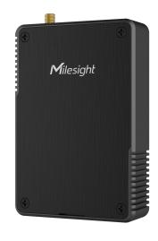
UG56 is a robust 8-channel indoor LoRaWAN<sup>®</sup> gateway. Adopting SX1302 chip and high-performance quad-core CPU, UG56 supports connection with more than 2000 nodes. UG56 has line of sight up to 15 km and can cover about 2 km in urbanized environment, which is ideally suited to smart building, smart industries and many other indoor applications.
