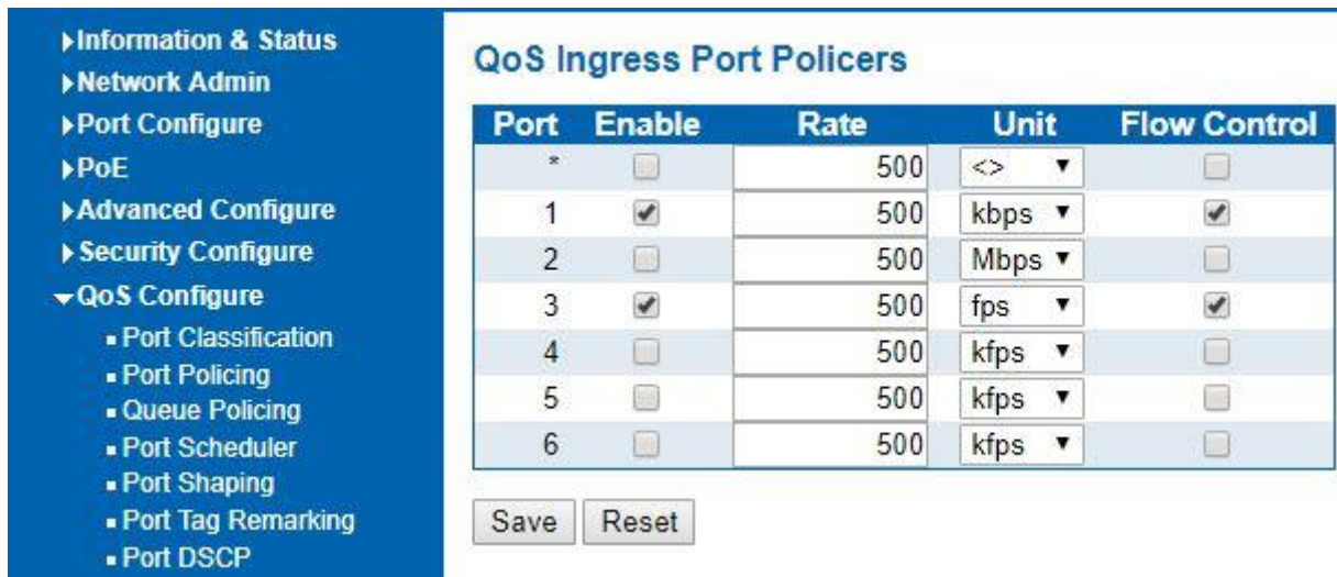
Figure 6-2 Port Policing Configuration Screen
