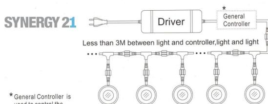
\* General Controller is used to control the RGB light.
