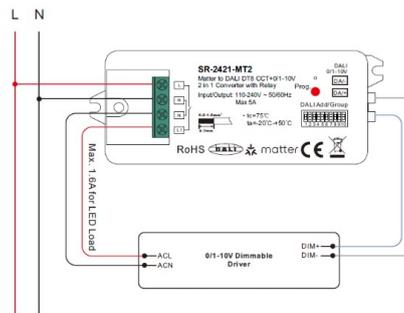
Note: the relay is only suggested to use when connected with 1-10V drivers which can not dim to off.
