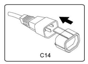
2. Insert the plug, with the Smart-Lock Plug Connector attached, into any available socket on a PDU by sliding it directly over and straight into the socket.
