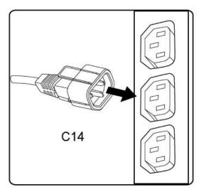
3. To disconnect the plug from the PDU, grip onto and squeeze the Smart-Lock Plug Connector as you pull and detach the plug from the PDU socket.
