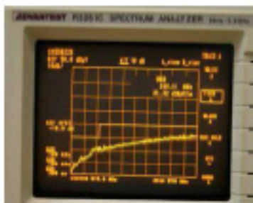
Radiated emissions measurement at 5W (max hold)
