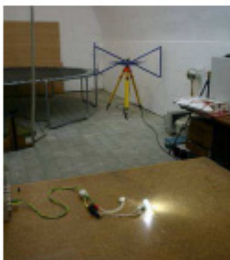
Radiated emissions measurement at 5W (max hold)
