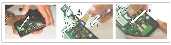
**Warning:** to avoid damaging the DIAL-103A or the SIM card, make sure that the unit is disconnected from power supply and from the RJ-11 connector before inserting or removing the SIM card. **Important tips for proper operation** We recommend to disable the PIN code request, voice mail, all call diversions (such as when busy, absent or not available) and call notifications on the SIM card before inserting the SIM in the DIAL-103A, using a normal GSM device with keypad.
