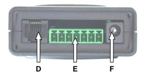
**D** = RJ-11 connector for a PBX trunk line interface or an analog telephone, pin 1-2-5-6 NC not connected, pin **3-4** connection for a PBX trunk line interface or an analog telephone.
