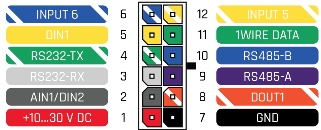
Figure 2 FMC125 2x6 socket pinout
