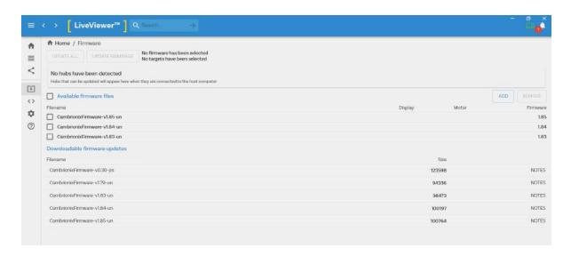
To install the firmware onto the hub simply click the hub/ hubs connected that you want to update and then select the firmware version you want to upgrade to. Once selected press the update button at the top and the update will commence.
