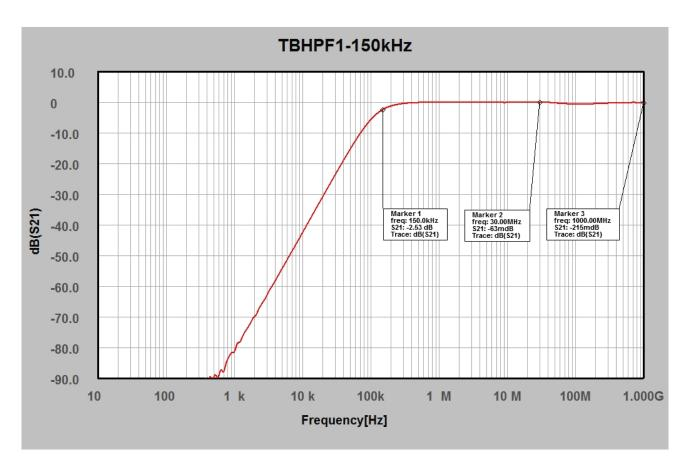
TBHPF1-150kHz: Attenuation 30 Hz to 1 GHz, typical data
