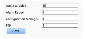
2. Set a priority level (0~63) for each service. At present, QoS allows you to assign different priority to audio and video, alarm report, configuration management and FTP transmission. The greater the value, the higher the priority. For example, if the value of audio and video is set to 60, alarm report and
