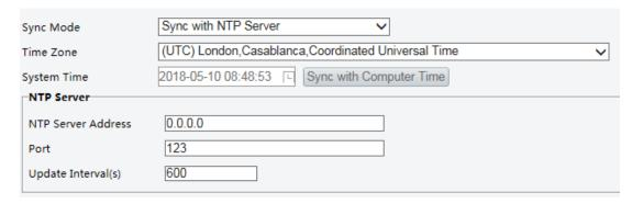
2. Set Sync Mode to Sync with NTP Server, and then set the IP address and port of the NTP server and update interval.
