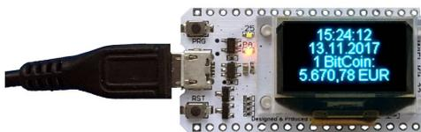
This product is an ESP32 module with a 4-pole OLED display. The module is delivered with a default software code. In order for this product/display to work according to your wishes, it must be loaded with individual software/Arduino code via a Micro-USB cable. Depending on which ready-made ESP32 Arduino examples you use from the internet or somewhere else, you may need to download the appropriate libraries so that the Arduino software can compile them for the Flash on the module.
