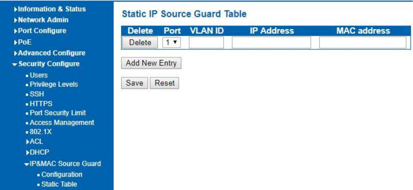
Figure 7-5 Static Table Configuration Screen
