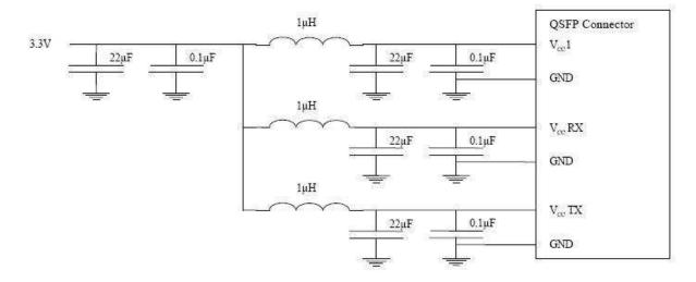
Figure 1. Host Board Power Supply Filtering
