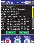
Capture up to 10,000 packets for analysis including packet size, source and destination IP address, time detected and packet type. User defined filters capture specific data needed to identify problems and monitor performance.
