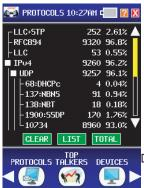
Lists all protocols detected with the total number of packets and the percentage of the total traffic. Certain protocols such as IPv4 and IPv6 can be expanded to show the sub-protocols.
