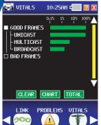
Vitals provides an indication of the operational condition of a network. A real time analysis a network. A real time analysis
