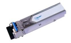
Wintop Small Form Factor Pluggable (SFP) transceiver is designed for data communication on Single-mode fiber and transmission distance up to 20km. The transceiver consists of five sections: the FP/DFB laser transmitter, the LD driver, the PIN photodiode, the limiting amplifier and the MCU control unit. And it compatible with Small Form Factor Pluggable Multi-Sourcing Agreement (MSA).
