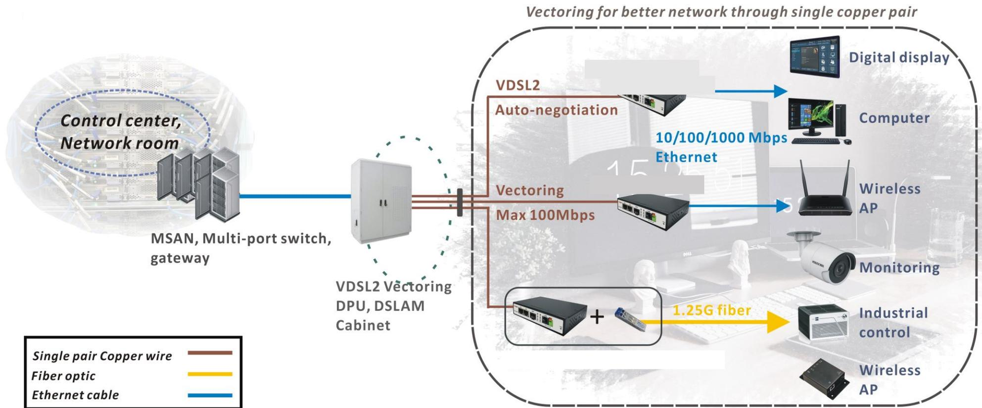
**Figure 2.2 Application Diagram**
