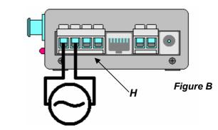
**Warning**: pin 2 of the "H" connector is connected to the **negative pole** of power supply: please keep in mind that anything connected to this pin will be referred to that negative.
