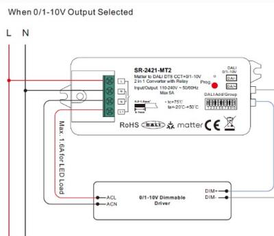
Note: the relay is only suggested to use when connected with 1-10V drivers which can not dim to off.
