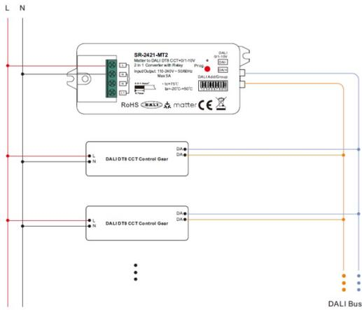
Note: Max. 50mA DALI bus PS output to supply control current to up to 25 control gears.
