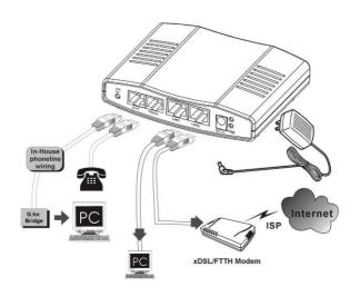
The figure above shows how to connect a FTTH/xDSL modem to a home phoneline network. Follow the same steps to connect any Ethernet device such as a STB or PC, to a home phoneline network.
