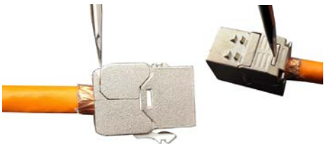
⑩.Press down the retainer for 360 degree shielding
